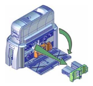
c. Load the overlay onto the cartridge. Make sure that the overlay spool color matches the cartridge spindle.
