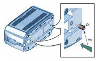
Return the laminator to its upright position and secure the laminator to the mounting surface with the two M6 screws.
