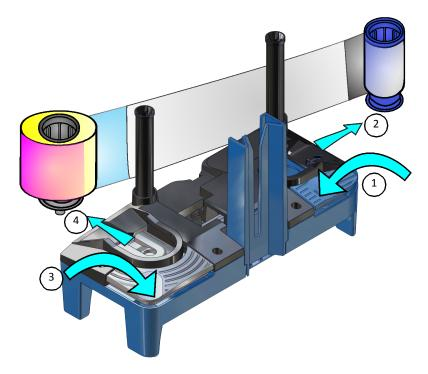
e. Remove the retransfer film from the film cartridge (C2).
