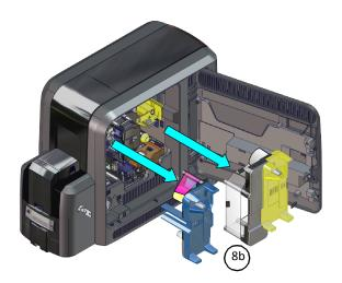
C. Remove the cleaning spindle (C3).
